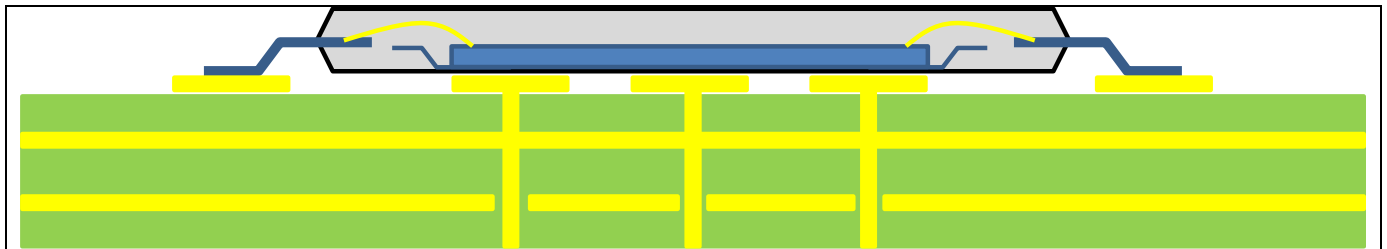
Figure 8-1: Example Thermal Via Holes on PCB
