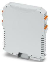
DIN rail housing, for mounting on a DIN rail, color: light gray (similar RAL 7035), width: 17.6 mm, height: 99 mm, depth: 113.65 mm, incl. 4 PCB connectors, 3-pos., screw connection, for 2.5 mm<sup>2</sup>, nominal current: 12 A, 320 V, PCB surface: 7500 mm<sup>2</sup>
